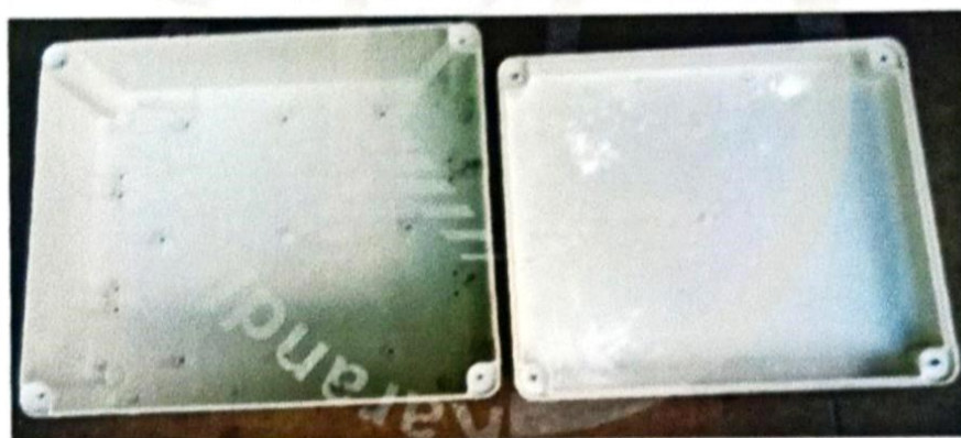
Picture2: No ingress of powder & water observed
