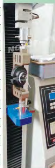
Novoflex Cable Ties are tested for specified Tensile Strength as per SAE-AS 3367
