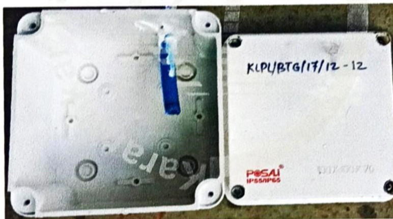
Picture2: No ingress of powder & water observed
